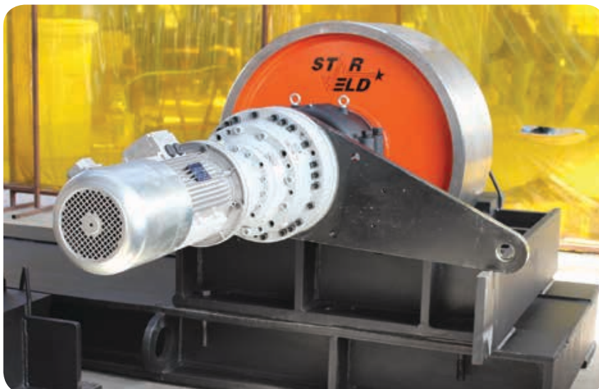
For the driven rolls, Bonfiglioli 7.5 kW induction motors connected to 311 planetary drives on a torque arm were chosen in a simple in-line design.
