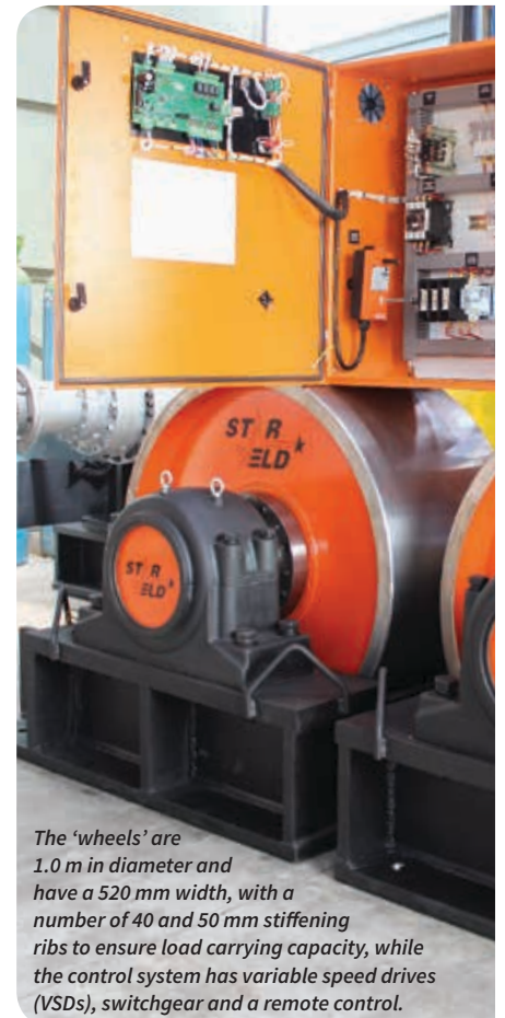
For the driven rolls, Bonfiglioli 7.5 kW induction motors connected to 311 planetary drives on a torque arm were chosen in a simple in-line design.
